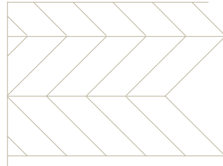
Figure 17: Fitting up against the wall.
