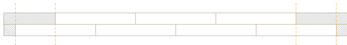
Figure 11: Gluing down initial rows with reference lines and fitted pieces.
